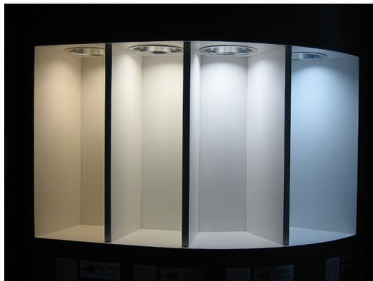
Color temperatures of white light varying 2700K, 3000K, 3500K, and 4100K from left to right. Image courtesy of ALG Online and the Energy and Technology Center.
